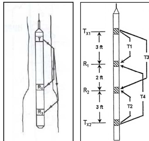
**Figure 1:** Schematic representations of dual receiver (CBL, left) and multiple receiver (BHCS, right) sonic tools. An open hole BHCS tool is two dual receiver type sonic tools stacked inline. Dual and multiple receiver type sonic tools are compensated for the effects of mud path contribution, eccentricization, hole deviation and washout.
