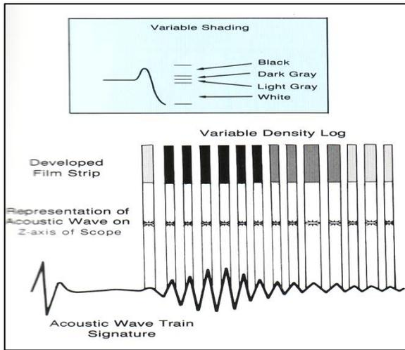
**Figure 2:** Representation of the acoustic waveform (bottom) transformed into a Variable Density Log (VDL) display (top) Positive amplitudes are black while negative amplitudes are white. Low amplitudes (including zero amplitude) are represented in shades of grey.
