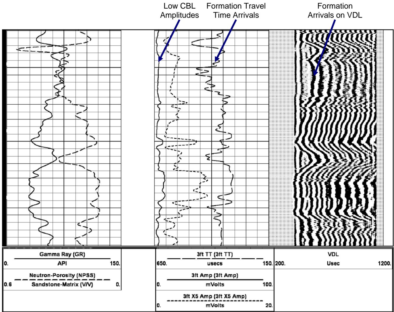
**Figure 6:** CBL-VDL-CNL log presentation obtained from RECON open hole BHCS with FWS function. Compensated Neutron (CNL) porosity on a sandstone matrix is presented with GR in Track 1. CBL Amplitudes and Travel Time are displayed in Track 2 with the VDL in Track 3. This section of log shows pipe with good cement bond; CBL 3ft amplitudes are low and formation arrivals are clearly visible on the VDL.
